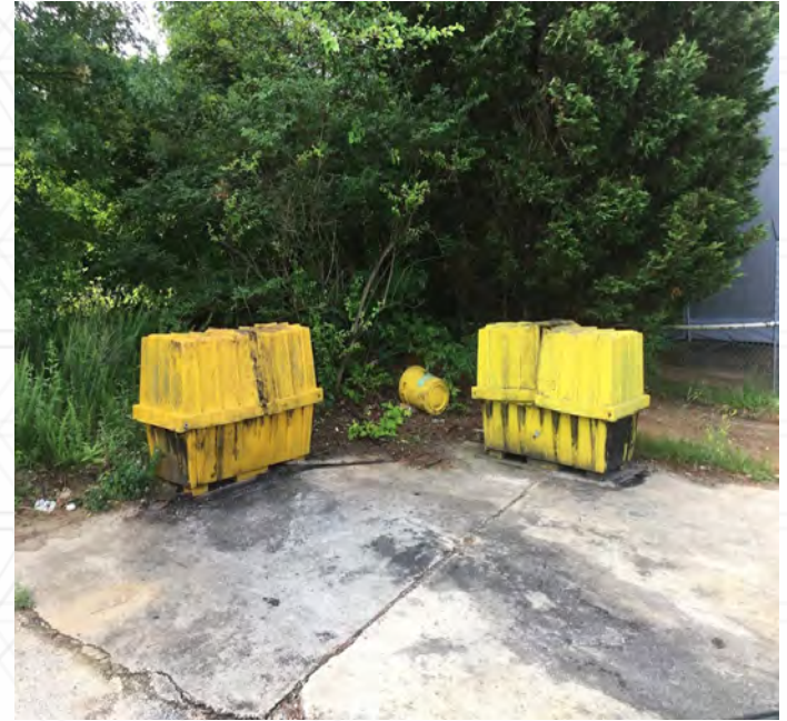
Containments are stained and have grease on the exterior, they are located in close proximity to the grassy areas, no spill kits.
